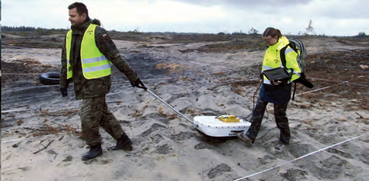
Research with geosonar, which allows to detect dangerous objects at greater depth. © Gmina Klucze
